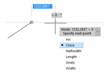
Dynamic input displays the command interface near the cursor in the drawing area. At the right time, current prompts, command requests, input fields, lists of selectable keywords, dimensions of edited geometry are displayed next to the cursor.
