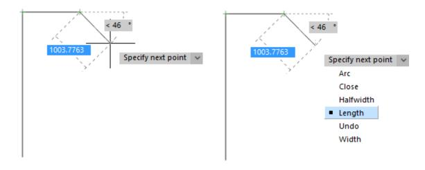
Dynamic input can be disabled by using a button in the status bar or by pressing **F12**.
