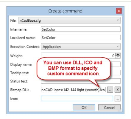
The standard technique for creating Lisp command involves: creating an LSP file, including it in the startup list of the **Load/Unload Applications** dialog, and only then, creating a new command in the **Customize User Interface** dialog.
