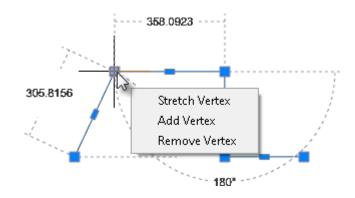
In the new version, the parameters of multifunction grips are available not only when the **CTRL** key is pressed repeatedly, they also appear in the pop-up menu when you place cursor on the grip.
