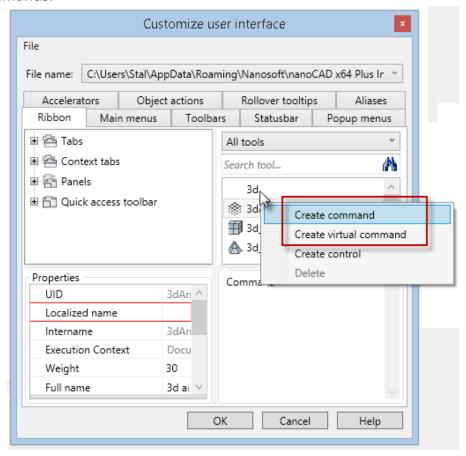
In nanoCAD 20 you can assign icons in ICO and BMP formats for custom and virtual command buttons.
