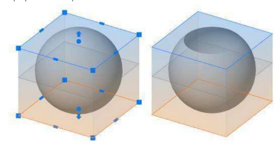
Drag grips to place the upper and the lower prism cutoff planes. Otherwise the upper and lower displaying area will be unlimited.
