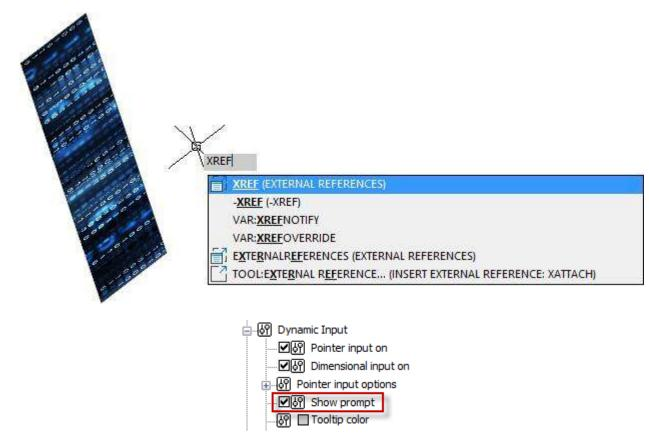
Dynamic prompts provide an alternative way to enter command parameter values. In the tooltip field near the cursor, requests and prompts of the active command appear, necessary to complete the command. Data can be entered in the dynamic prompt fields instead of the command line. You can enter command keywords and requested numeric values.
