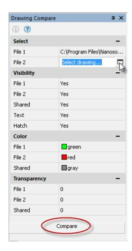
The Compare Files (DWGCOMPARE) command (the Functional Bars section on the Options tab) displays a functional panel with settings and a launch button.
