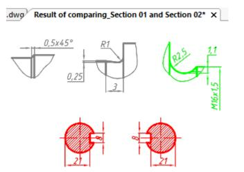
The feature creates a new dwg file that displays similar and different objects of the compared files, coloring them in several colors. In addition, you can switch off the displaying of unnecessary
