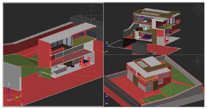
An existing prism can be changed, deleted or disabled/enabled. If the prism is disabled, graphics outside the prism become visible. Disabled prism object is still present in the model space and can be switched on later.
