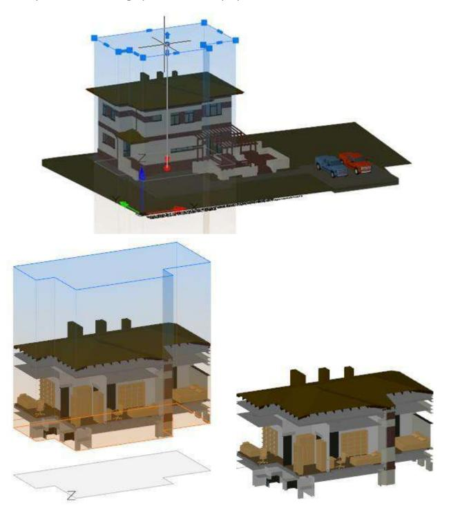
The area is defined as a rectangular or polygonal prism with grips. The prism can be:
