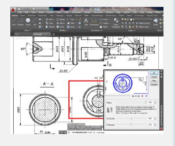
In WiseImagefor AutoCAD tools it is possible to crop, change resolution, scale, deskew, and calibrate colour and greyscale raster images. It is possible to change brightness, contrast, hue and saturation and adjust the colour gamut, improve image quality and apply colour. Users can rasterize vectors to generate ISO compliant raster as often required for compliancy purposes. Merging monochrome and colour images is also a one-click task.
