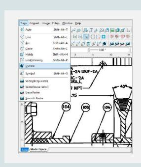
Select a raster shape and WiseImage will automatically match it to the appropriate vector object from a default Symbol Library or a customized library created to match user requirements. The polyline tracing feature includes auto detection of tracing direction.
